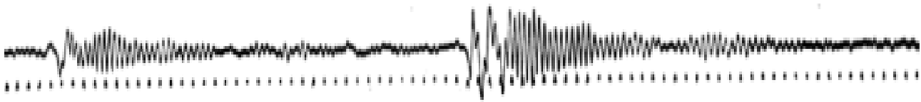
Figure 32: Early records of tweaks (oscillogram of tweaks) and the timing impulse frequency, 1000 Hz. Adapted from [Burton and Boardman, 1933].
